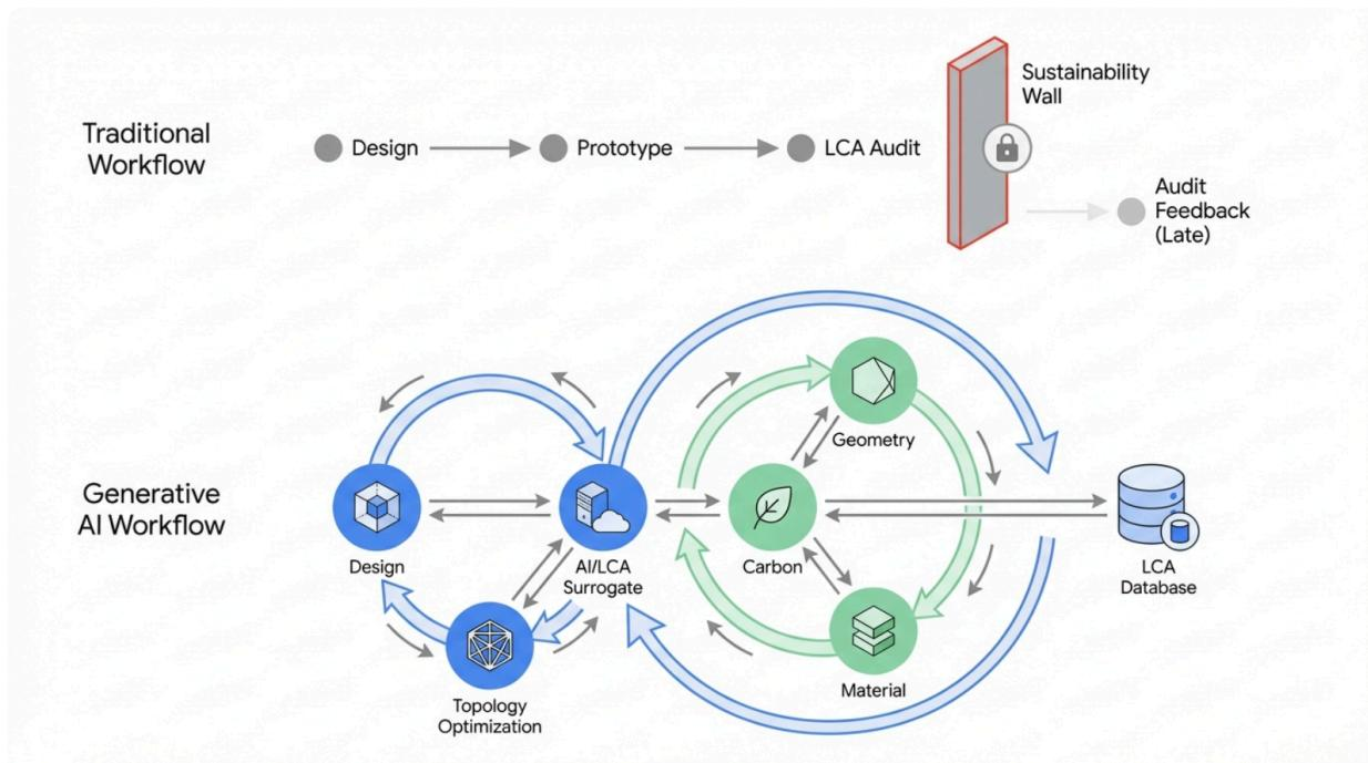
Comparison of the traditional manufacturing workflow, where sustainability is audited after design freeze, versus the Generative AI workflow, where surrogate models and topology optimization provide real-time carbon feedback during the ideation phase.
