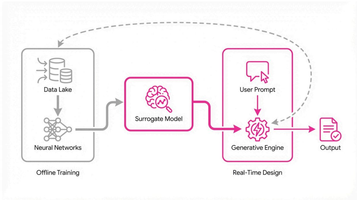
Schematic of an AI-driven Predictive LCA framework. Historical LCA and geometry data (left) train the Machine Learning Surrogate Model. This model is then embedded into the Generative Design Engine (right), providing millisecond-level carbon estimates to the optimizer.
