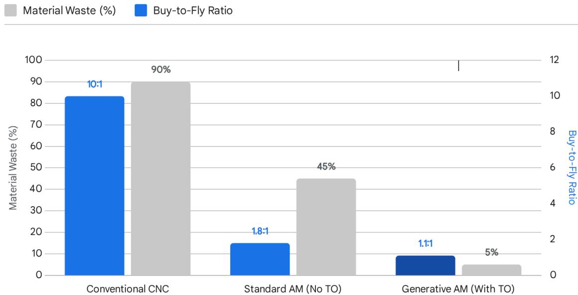
Comparison of material waste percentages and buy-to-fly ratios between Conventional Machining (CNC) and Generative Design coupled with Additive Manufacturing (AM). Data indicates waste reductions of up to 90% and significant improvements in material utilization ratios.
