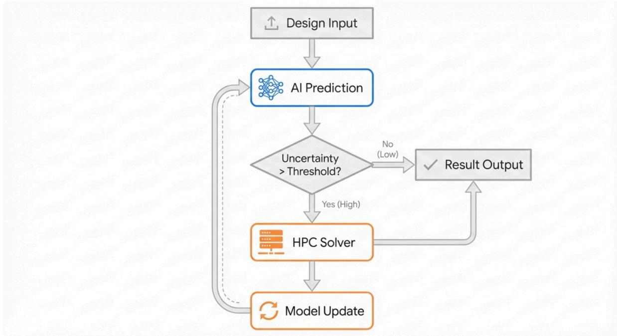
The adaptive agentic workflow for physical simulation. The agent primarily uses a Large Physics Model (LPM) for near-real-time design evaluation. However, an 'Uncertainty Monitor' acts as a gatekeeper; if the design falls outside the model's confident training distribution, the agent autonomously dispatches a job to a traditional High-Fidelity Solver (CFD/FEA) to validate the result and retrain the model.
