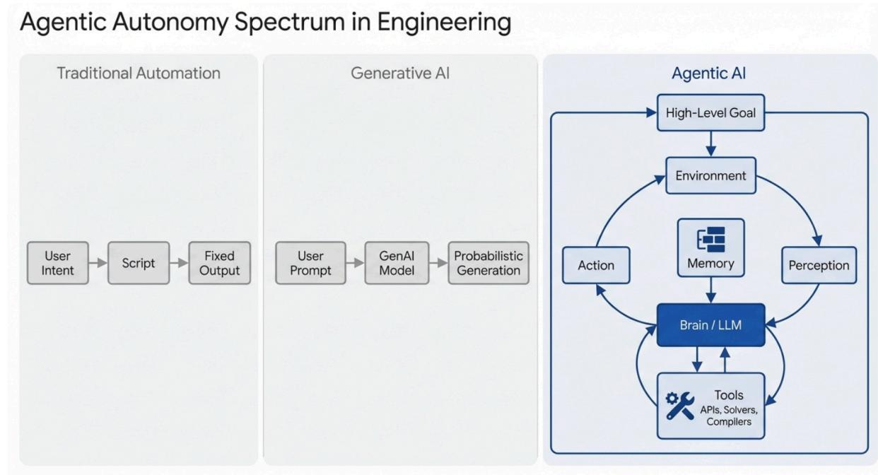
The evolution of engineering tools from passive instruments to autonomous agents. While traditional CAD and Generative AI rely on explicit user triggers for every step, Agentic AI introduces a recursive 'Reasoning and Acting' loop, allowing the system to decompose high-level goals into sub-tasks and execute them using external tools.
